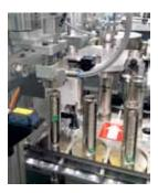
Bimetal magazine on the automatic feed with ring and core blanks
