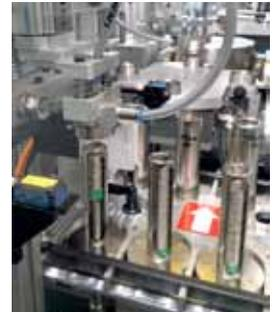
Bimetal magazine on the automatic feed with ring and core blanks
