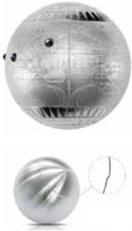
Blank made of rough-turned silver. The sphere was made with excess material. The trick was to precisely dimension this excess material.
