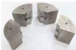
The complete tool consisting of four segments and a pair of coining dies.
